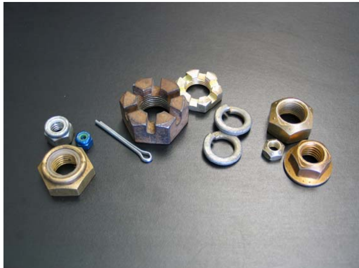
Figure 9 – From left: nylon collar lock nuts, castellated nuts, spring lock washers, flanged and non-flanged deformed thread lock nuts
