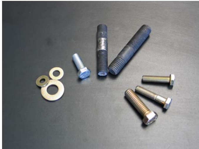
Figure 3 - Clockwise from left: Grade 8 flat washers, Grade 5 UNF bolt, UNF/UNF stud, UNC/UNF stud, Grade 8 bolts
