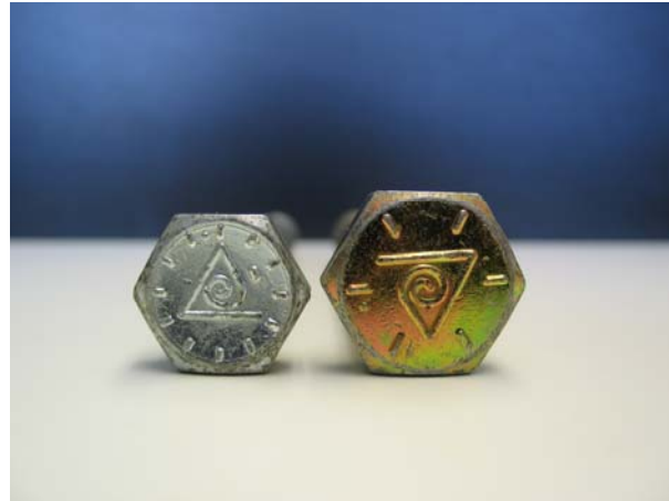
Figure 7 - Bowman Grade 8 bolt & Bowman “Special Alloy” bolt
