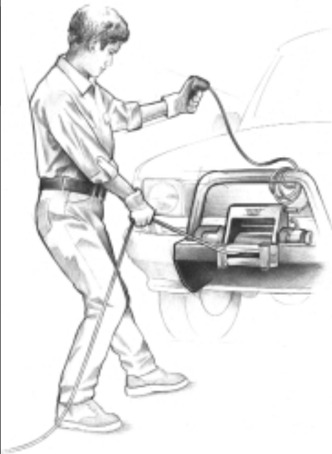
Step 19: REWIND WIRE ROPE. The person handling the wire rope should walk the rope in and not let it slide through the hand and control the winch at all times.
