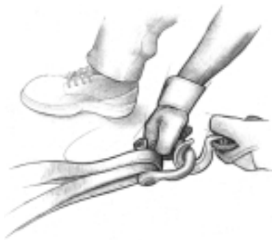
Step 18: DISCONNECT WIRE ROPE. Disconnect from the anchor.
